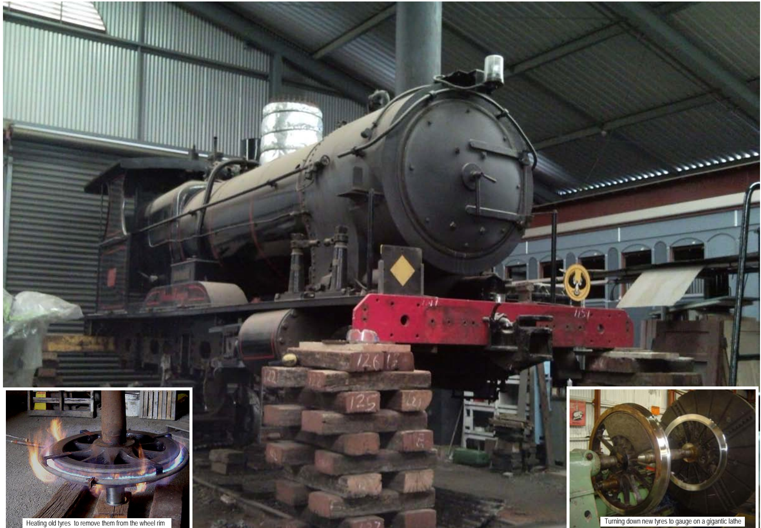
Heating old tyres to remove them from the wheel rim
